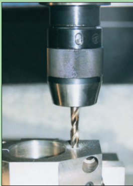
1 Drill coolant passage, leaving reaming allowance.
