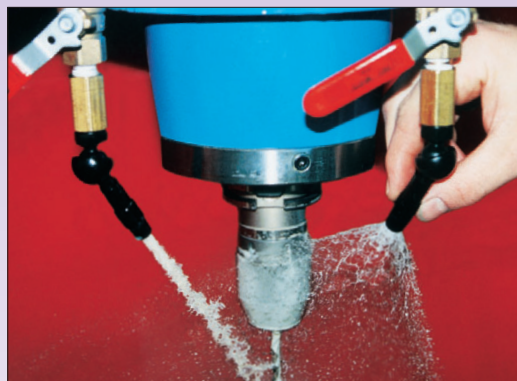
MillJets shown installed on Vertical Machining Center showing wide and narrow spray.
