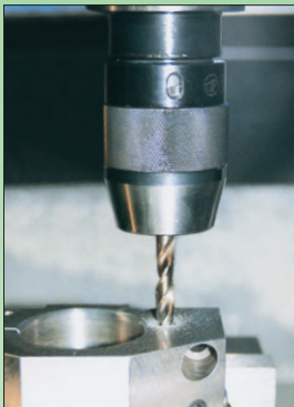
1 Drill coolant passage, leaving reaming allowance.
