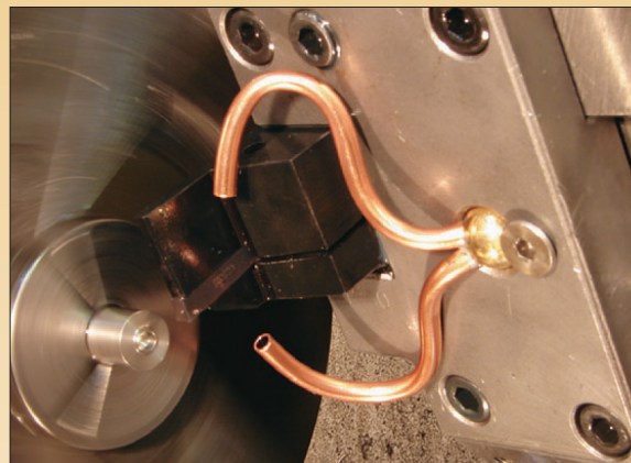
TwinPop nozzle shown installed in lathe turret.
